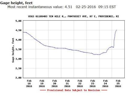
**Important note:** The gage reading at this time was 4.51 feet. Typical of many streamgages, this is <u>not</u> the actual elevation above sea level, but instead is based on the size of the gage itself. To convert the gage reading to height above sea level, add 9.84 feet to the gage height.
