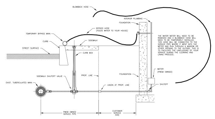
Figure 1 - Typical "Temporary By-Pass Piping" Installation
